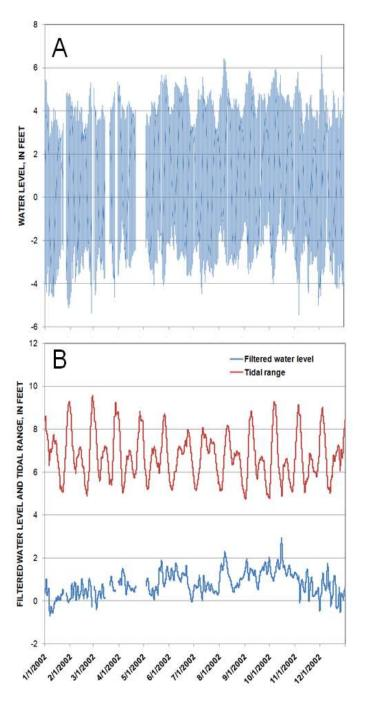
Figure 3. Decomposition of the Fort Pulaski (station 02198980)15-minute water-level signal (A) into the periodic component of tidal range and the chaotic component of daily water level (B).
